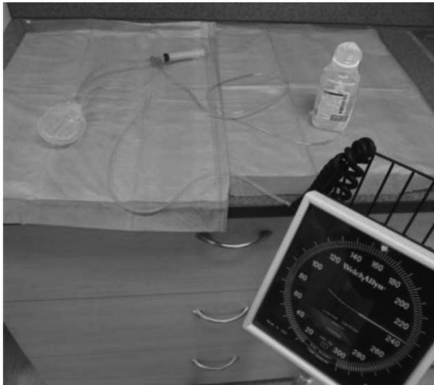
**Figure 3.** After removal of the air from the drain reservoir, one of the two ports on the top was connected to tubing with a three-way stopcock, allowing for saline to be injected into the drain reservoir in known volumes. The second port was connected with similar tubing to a sphygmomanometer to measure the suction of the drainage system.
