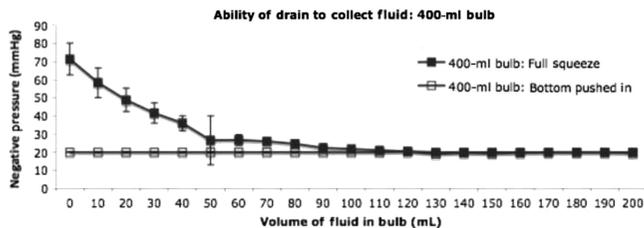
**Figure 5.** Using a 400-ml Jackson-Pratt drainage system, average suction was measured using either the full side-to-side squeeze or the bottom-pushed-in technique of generating negative pressure. Measurements were repeated five times and means were reported  $\pm$  the standard deviation.
