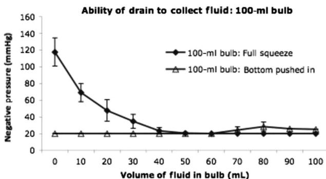
**Figure 4.** Using a 100-ml Bard drainage system, average suction was measured using either the full side-to-side squeeze or the bottom-pushed-in technique of generating negative pressure. Measurements were repeated five times and means were reported  $\pm$  the standard deviation.
